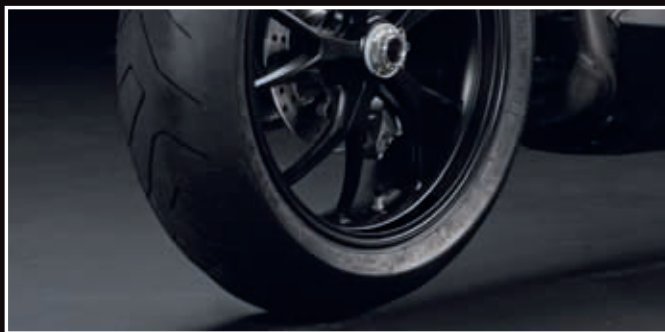
La 848 monta pneumatici Pirelli Dragon Supercorsa PRO 120/70 ZR17 all'anteriore e 180/55 ZR17 al posteriore. / The 848 uses Pirelli Dragon Supercorsa PRO tyres. Sizes are 120/70 ZR17 front and 180/55 ZR17 rear.
