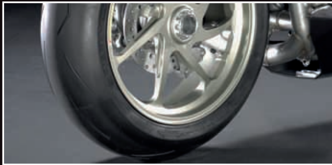
Il modello 'S' monta pneumatici Pirelli Diablo Supercorsa SC 120/70 ZR17 all'anteriore e 190/55 ZR17 al posteriore. / The 'S' uses Pirelli Diablo Supercorsa SC tyres. The sizes are 120/70 ZR17 front and 190/55 ZR17 rear.
