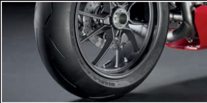
La 1198 monta pneumatici Pirelli Diablo Supercorsa SC 120/70 ZR17 all'anteriore e 190/55 ZR17 al posteriore. / The 1198 uses Pirelli Diablo Supercorsa SC tyres. The sizes are 120/70 ZR17 front and 190/55 ZR17 rear.
