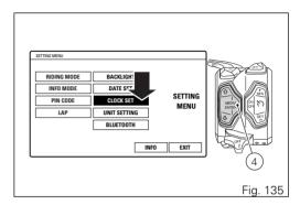
When entering the function, available settings are indicated on the left: HOUR, MINUTE, AM / PM, while set time is indicated on the right (e.g.: 10 : 30 a.m.).
