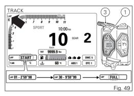
If the LAP function is not selected from the menu, the instrument panel will go back to the functions present before the FLASH button (3) was pressed.
