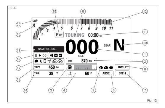
Data displayed on the main screen for CORE layout are as follows:
