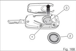
Install the battery in place, paying attention to respect polarity: positive pole (+) must be facing up.
