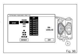
When entering the function, the currently set DTC level or status is indicated on the right (e.g.: ON LEVEL 03).
