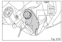
This type of mixture ensures the best operating conditions (the coolant starts to freeze at -20 °C/-4 °F). Cooling circuit capacity: 2.5 cu. dm (litres).
