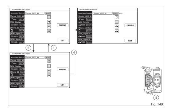
To pair a Smartphone, the pairing procedure with the Bluetooth control unit requires user to enter a code (0000), which is only necessary the first time the device is paired with the Bluetooth control unit. In this case, the Instrument panel displays the PIN to be entered "INSERT PIN ON SMARTPHONE: 0000". When user enters the PIN on the Smartphone, the device will be paired.
