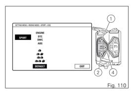
It will take three seconds to restore parameters, during which "WAIT..." will appear on the display. Once procedure is completed, "OK" will appear for two seconds to confirm that default parameters have been restored and the message EXIT will be highlighted.
