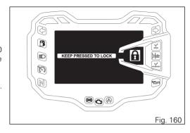
Warning reading "Steering locked" (upon Key-Off)
