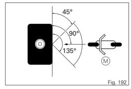
In this case it is not possible to provide protection against the first impact (on the road), since the activation logic detects the skidding or fall condition and the airbags are inflated completely only after the rider and/or passenger hit/s the road.
