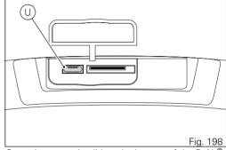
Open the protection lid on the bottom of the D-Air® installed in your jacket/waistcoat, find the USB microport (U) and connect the battery charger cable. At the beginning of the recharging phase, 4 LEDs turn on in sequence to indicate that the recharging is in progress. When the battery is charged, 4 green LEDs will be steady on. Disconnect the battery charger as soon as the recharging process is completed. The system complete recharging usually takes approximately 4 hours.
