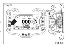
When SET button (7) is pressed, current speed is set as target cruise speed.
