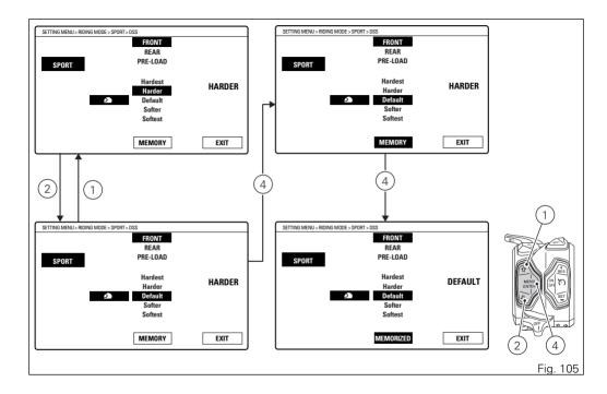
Adjustment of rear suspension rebound and compression damping
