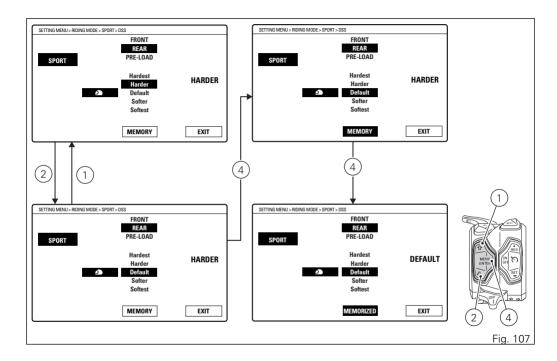
Adjustment of the rear shock absorber spring preload
