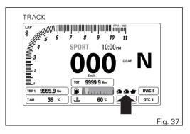
Note In case of system fault, set setup symbol will be ORANGE.
