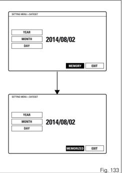
If date is not correct, the instrument panel will display "WRONG DATE" flashing for three seconds and then will automatically highlight EXIT, while date is indicated as "---/-/-" steady. It is still possible to set a new date.
