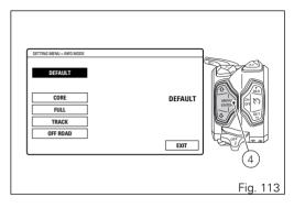
To select a layout for all riding modes, press button (1) or button (2). Once mode is highlighted, press button (4). The selected option is stored, current mode indication is refreshed and the EXIT option is automatically highlighted.
