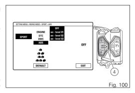
When entering the function, the currently set ABS level or status is indicated on the right (e.g.: OFF). Customisation options are indicated on the central drop-down menu: levels 1 to 3 and status OFF. Press buttons (1) and (2) to highlight the levels one by one: in particular, use button (1) to highlight the following item and button (2) to highlight the previous item.
