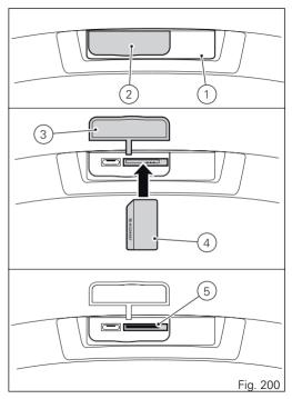
Pairing procedure of the D-Air® device present on the Jacket/Waistcoat with the bike D-Air® system.
