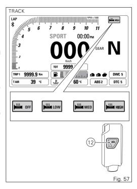
Level selection with Heated Handgrips "off": Even if heated handgrips are turned off, it is still possible to set them to LOW, MED or HIGH level, but the icon will have a white background (in DAY backlighting option of the instrument panel) or BLACK (in NIGHT backlighting option of the instrument panel).
